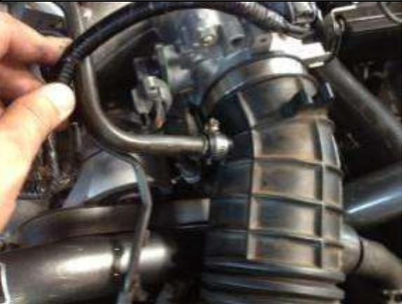
c. Re-connect the vent tube and secure with the clamp.
