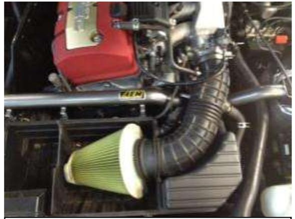
b. Re-install the intake tube/air filter assembly.
