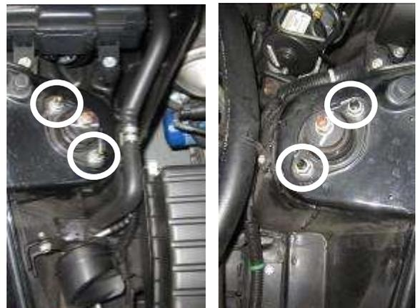
d. Remove the 4 damper nuts.
