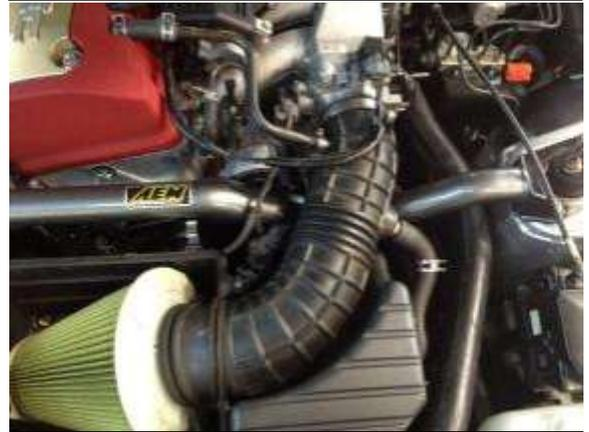
d. Re-connect AIT sensor wire, clip sensor wires back to intake the intake tube.
